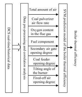
Fig. 1. Prediction model structure of boiler thermal efficiency
